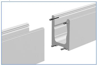
3 Position base rail and secure bolts with torque.
