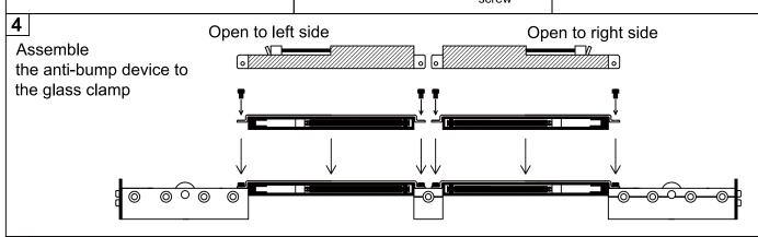
Fix the glass clamp with anti-bump device to glass panel
