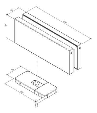
Self closing floor mounted patch fitting for Frameless Glass Doors & Pool Gates.
