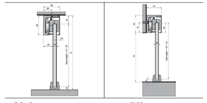
Ceiling fix To determine door height H = Overall opening height DH = Glass door height DH = H less 37mm
