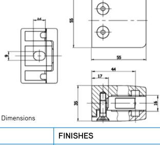
Balustrade Clamp with Retaining Plate - Flat back for square post or wall mounting Polished Suitable for 10 & 12mm toughened glass Satin Can be friction fit and/or firmly secured with retaining plates on the top & Matt Black bottom of the glass panel
