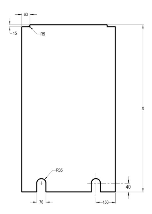
X = height of door which is finished opening height less 35mm
